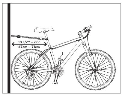
6. Max load weight on the Bike Nook (Telescopic) is 66 Lbs (30 Kg)
